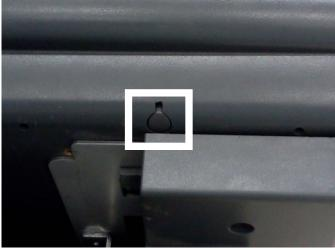
To reboot the workstation using the power button simply hold the button down for approx 10 seconds. Once the workstation is off push and release the power button.
